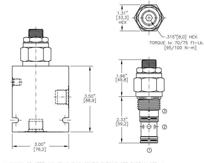
FOR ALUMINUM OR STEEL VALVE HOUSING CONFIGURATIONS SEE PAGE 0-023-1.
